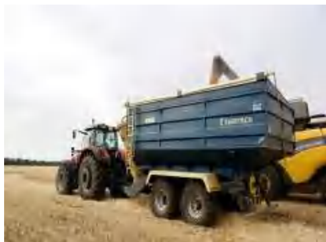
Fig. 1 Agrotech storage and reloading bunkers [1].
