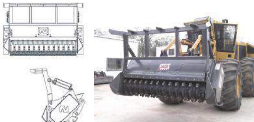
Figure 2. – Hydraulically driven Nokamic mounted mulcher (Canada)
