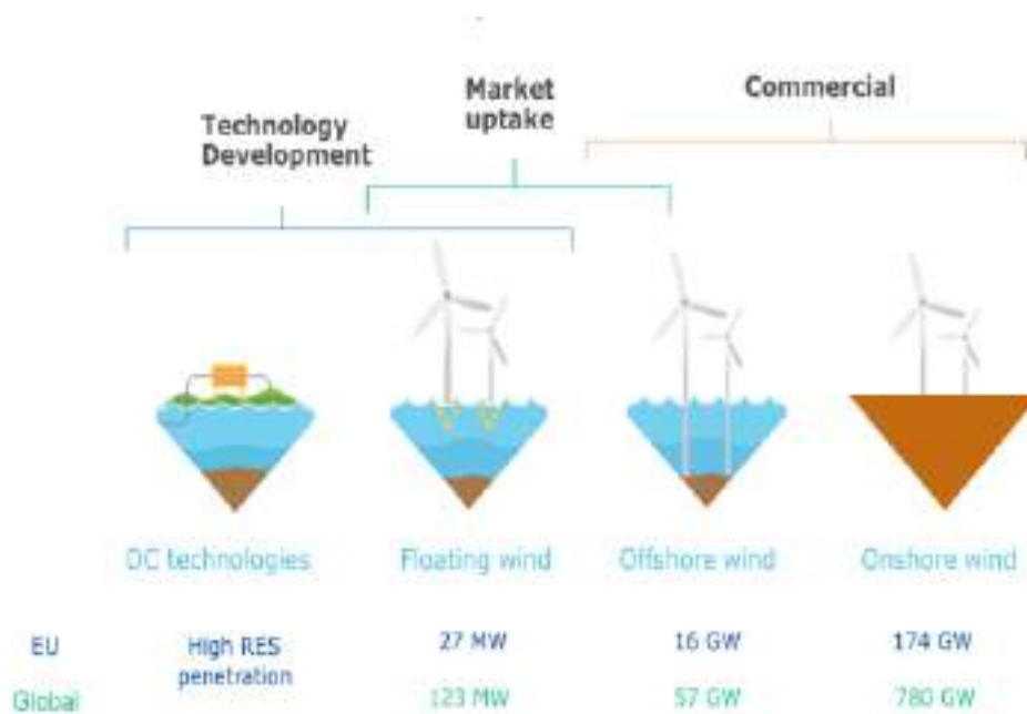
Fig. 1. The level of technological readiness of the main technologies in wind energy and installed capacities in the EU and the world in 2021 of wind energy generation technologies.
