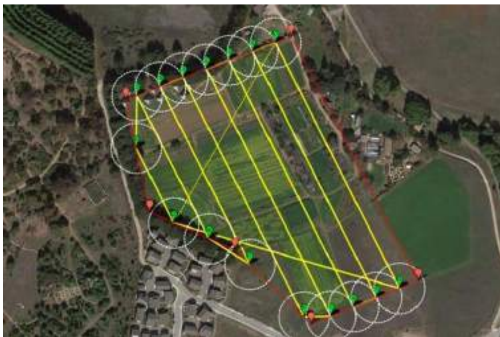
Fig 4. An example of a UAV flight route when planning a terrain survey Use of optoelectronic means
